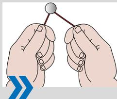
Thread the safety wire through your fastener(s) in the appropriate manner. You will now have two ends of the wire ready to twist.
