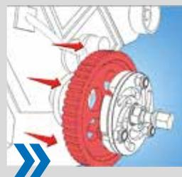
When finished working, remove puller.
