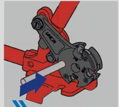
1. Insert the threaded rod into the opening of the corresponding dimension.
