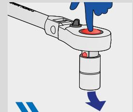
The socket is be released from the ratchet by simple pressing the button.
