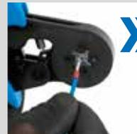
➤ High-precision die geometry leads to a clearly defined crimp shape of the ferrule.
