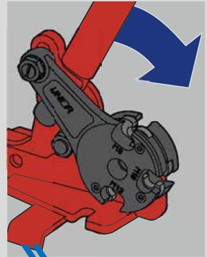
To operate correctly, the cutter should be opened by raising the top lever handle to its maximum extent. When it is fully open, insert the threaded rod into the cutter opening of the corresponding dimension.
