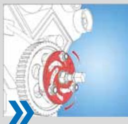
Turn setting plate to shift puller legs, so they tightly grasp to pulley.
