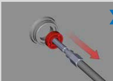
▶▶ After several strokes fast and easy dismount bearing from housing without damage.
