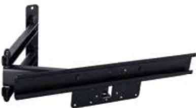
► Foldable small parts organizer mounts to the Unior work bench support and provides optimal placement for it. The setup will make work more comfortable and productive as the smaller parts will be right where you need it. Parts organizer can be rotated 90° left or right, foldable arm is 500 mm long and allows to pull the organizer or fold it out of work area when not in use. Organizer is compatible with all sizes of plastic boxes in our range.
