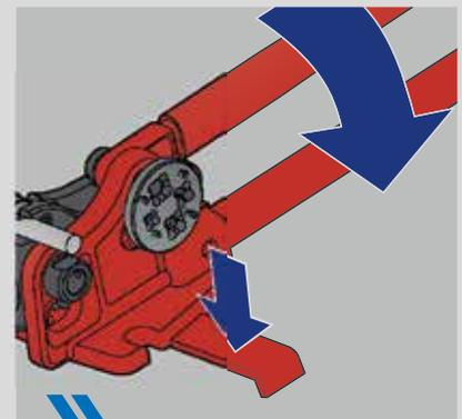
Important notes when cutting! When operating on the floor, apply foot pressure on the bracket.
