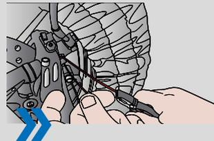
Use the safety wire twisting pliers to grip the two wires at an appropriate distance from the fastener. The length of wires between the pliers and the fastener will be twisted in the following step.
