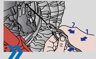
Slide the central chromed locking sleeve to lock the plier handles together, clamping the wire ends.
