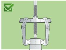
*Always centre the puller spindle on the middle of the object, so the holding arms are distributed evenly on the body.*
