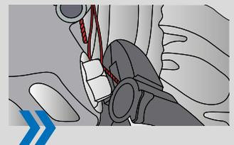
Squeeze the plier handles to release the chromed locking slider, and then use the integrated wire cutter to trim the wires to length.
