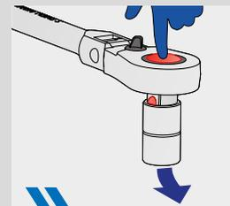
The socket is released from the ratchet by simple pressing the button.
