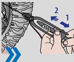
Let go of the plier handles and pull the chrome handle at the base of the pliers to rotate the pliers and twist the wire in a clockwise direction.
