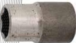
**2. CNC working of the socket:** A special-purpose CNC machine is used to work the socket into the required size according to the ISO standard.
