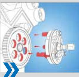
Insert puller legs into openings of pulley.
