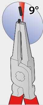
The tips are inserted into the jaw at an angle that prevents the circlip from sliding off the tips.
