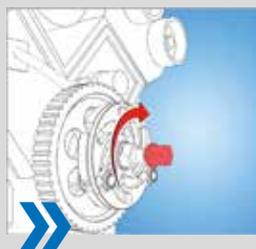
Turn spindle clockwise until pulley comes off.
