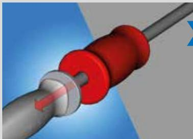
▶▶ Start with steady hits dismounting bearing with help of sliding hammer.
