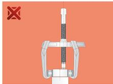
*Never put the puller spindle off centre, as slippage of the puller arm can occur.*
