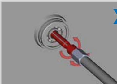
▶▶ First inserted extractor through the hole in the bearing which will be dismount out of the housing. Then start to screwed thorn into extractor, which has a function that opens puller body, which adapts to the bearing bores.
