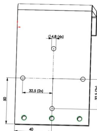
Drawing for drilling, cut four M6 threads
