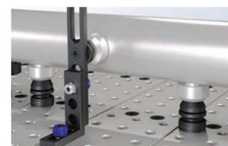
Vertical application using Locating Post + V-Block Spacer
