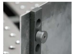
Magnet keeps sheet metal in vertical position
