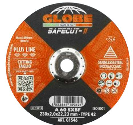
The **SAFECUT** series by Globe consists of thin discs that are extra rigid due to the metal safety ring. The result is a highly stable disc without vibrations. The 115mm and 125mm discs feature a ring of only Ø55mm, allowing for maximum utilization of the disc.
