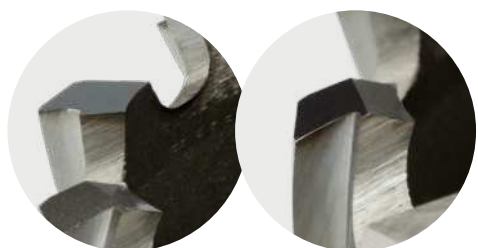
HSS cutters have two different teeth
