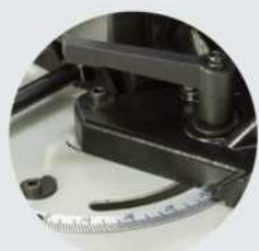
Wide cutting angle adjustment range
