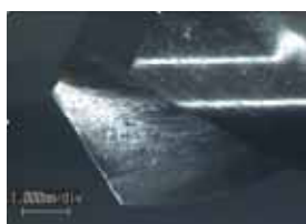
Small wear after drilling 10400 holes
