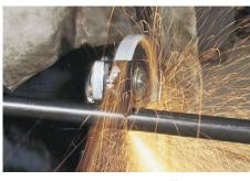
X-Cellence ONE: ultra-subtle cutting disc with a very high life. The depressed center "narrow dome" allows a bigger cutting penetration and a high number of cuts.
