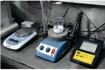
PH metric titration of resin powder.
