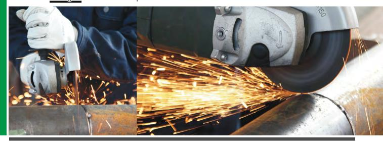
**PIPELINER** is the cutting, grinding and beveling range designed for pipes fitting, notching and welding preparation. These discs are specially formulated and reinforced for grinding joint welds between passes in pipeline construction. Free from Iron, Sulphur or Chlorine (Fe, S, Cl), they don't contaminate stainless steel.
