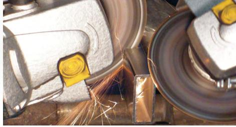
**COMBI SPEED** swas especially conceived by GLOBE for cutting and light grinding or beveling with one single product. COMBI SPEED is the evolution of COMBI wheel and thanks to the 2,0 mm thickness only and the 2-layer structure with 3 reinforcement cloths, it combines in a single disc an excellent cutting capacity and high safety during grinding operations. Safety and resistance of COMBI SPEED are constantly internally tested by side-load tests and burst test.
