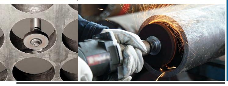
These wheels are generally used on portable straight grinders for internal grinding of workpieces, such as internal lapping of pipes in the petrochemical industry. Great care is taken in balancing these wheels to prevent vibrations
