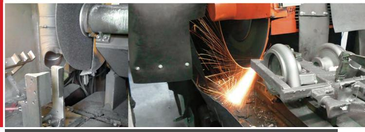
GLOBE cutting discs for stationary machines offer a wide range of products for cutting the most different types of materials and are available in diameters from 300 mm up to 800 mm with thicknesses that vary from 3 to 9 mm. There is also the possibility to change the bore size according to customers' needs. Particular care is taken in balancing these discs to obtain a product without vibrations..
