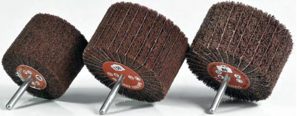
Non-woven **FLAP WHEELS** composed by Corundum and non-woven+abrasive canvas with 6 mm shaft. These are similar to the non-woven wheels, but with the addition of the abrasive canvas, it allows a better removal eliminating the possible scratches left on the processed object.
