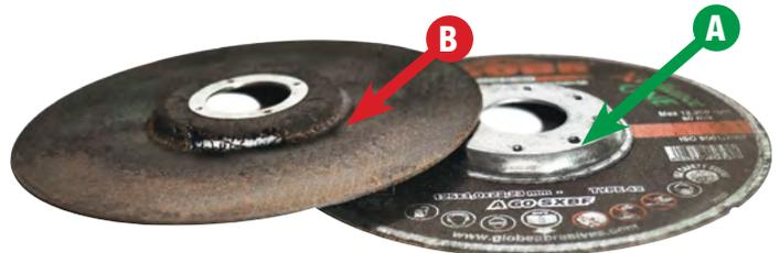
Thanks to the use of the special **"SPACER"** and to the depressed center shape, the machine shaft and the locknut do not stick out from the dome cavity, enabling the operator to carry out flush cuts in a comfortable position. The depressed center shape gives more rigidity than a flat disc, prevents bending allowing to make perfectly straight cuts.
