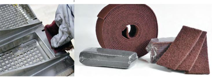
**NON WOVEN PADS** and **ROLLS** are used for hand works or mounted on orbital or rectilinear polishers. With this type of extremely versatile product that is available in the Aluminium Oxide and Silicon Carbide versions, it is possible to work in an excellent way on a wide variety of surfaces: steel, iron, metals, wood, plastic, ceramic.
