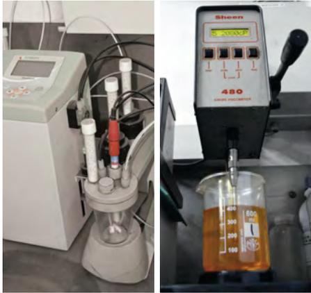
Titration of chemical compounds. Determining the viscosity.
