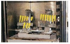
Scroll test for phenolic resins powder.
