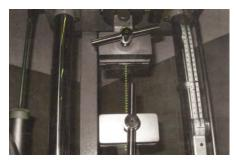
Yarn resistance test of the strengthening nets.
