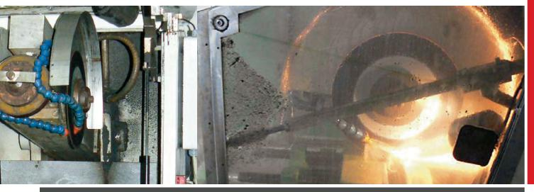
Built with reinforcements for cutting test pieces exclusively with enclosed machines. Also with coolant. Thanks to the high cutting capacity they do not overheat the workpieces and allow a precise, fast and cold cut. Available in diameters 250,300 and 350 mm, their mixture does not contain iron, sulphur and chlorine compounds.
