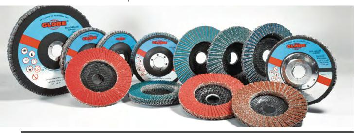
Flap discs with fiberglass backing pads have the special feature of not dirtying with plastic material stains. This phenomenon can occur when the abrasive cloth is almost worn out and, unwittingly, the plastic pad rubs against the metal. This requirement is particularly important when working on stainless steel.
