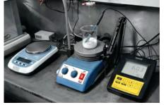
PH metric titration of resin powder.
