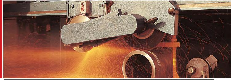
These cutting wheels can be used effectively in a variety of applica- tions in foundries, with ferrous and non-ferrous metals.
