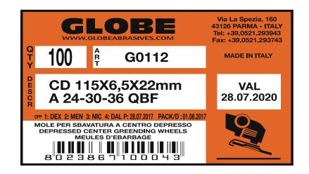
**For each single GLOBE wheel**, at the moment of manufacturing, an individual label is prepared showing day, month and year of expiry (the same as those of manufacturing but with 3 years more) as well as identity of the operator in charge of pressing. Labels are prepared through a special machine connected to the central computer system.
