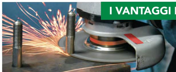
Flush cut possible thanks to the depressed center shape and the use of the "SPACER".
